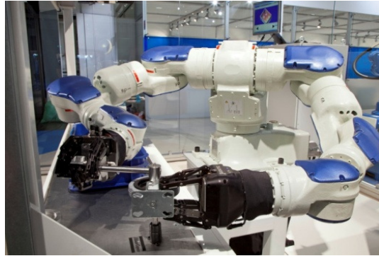
SDA20D in combination with adaptive grippers and 3D image processing software
